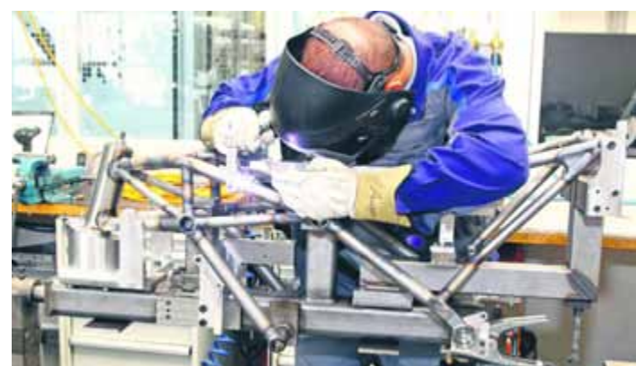
Work is underway on welding the C-01's cro-moly steel frames
